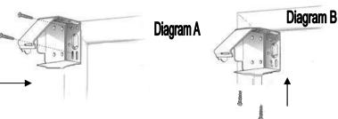
(Diagram B) position top of bracket against inside surface of window frame and attach as shown. Each end bracket uses two screws mounted diagonally. Make sure end brackets are level.
