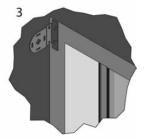
3) Fit control end bracket at the left hand side
