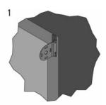
1) Starting at the right hand side, place and secure a control end bracket at the measurement taken
