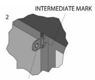
OUTSIDE FACE OF INTERMEDIATE BRACKET (MUST BE IN LINE WITH INTERMEDIATE MARK)
