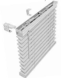
the bracket against inside surface of the window frame and fasten by screwing in screws through top holes in bracket. Each end bracket uses two screws. The screws mounted diagonally. Make sure end brackets are level.
